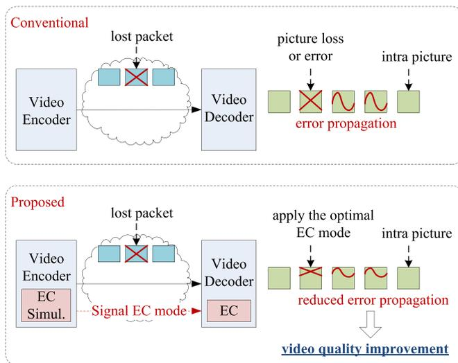
Fig. 2. Conceptual diagram of the EC mode signaling to reduce the error propagation (upper: conventional method, lower: proposed method). (For interpretation of the references to color in the text, the reader is referred to the web version of this article.)
