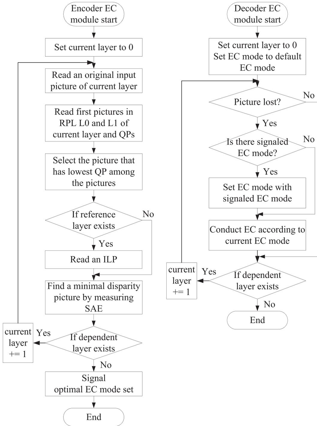
Fig. 3. (example) EC mode signaling algorithms of an encoder (left) and a decoder (right).
