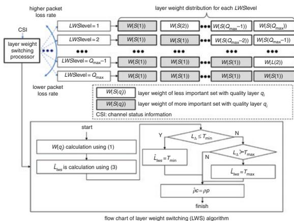
Fig. 1 Schematic illustration (upper part) and block diagram of the proposed LWS method
