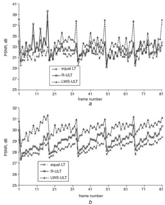
**Fig. 4** PSNR comparison of the proposed LWS-ULT with equal LT and R-ULT for different packet loss rates and video sequences
