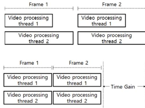
**Fig. 3.** Example of the decoding time gain from considering asymmetric performance ratio of big/little cores
