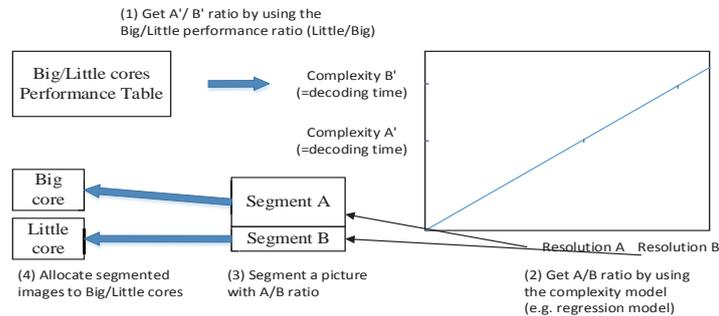
Fig. 4. The procedure of proposed method
