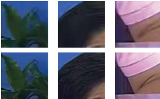
Fig. 11: Reconstructed image comparison with enlarged noticeable sections: (upper) EC mode 2, (lower) EC mode 4 (proposed method).
