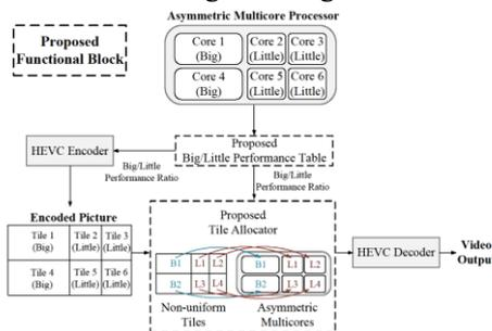
Fig. 1 Block diagram of the proposed HEVC encoding/decoding system
