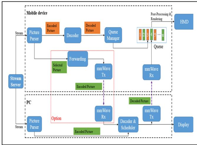
Fig. 6. PC Offloading mechanism
