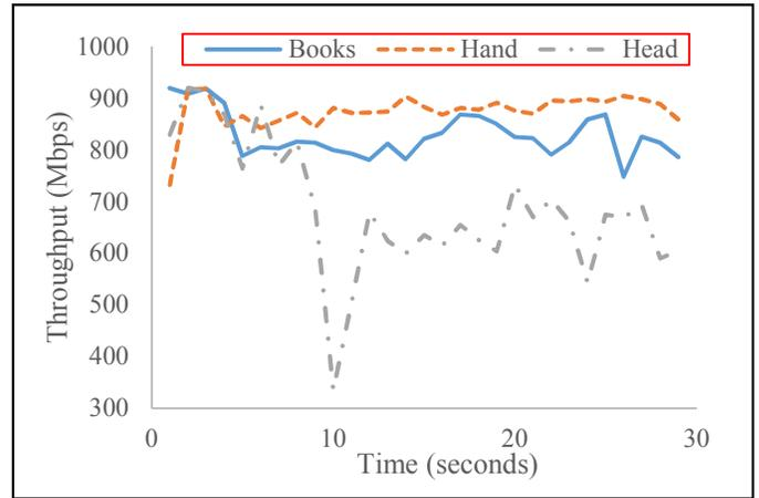
Fig. 9. The data rate of mmWave connection effected by obstacles
