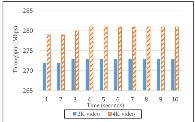
Fig. 10. Throughput of mmWave link for real-time video streaming
