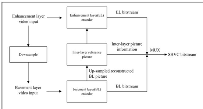
Fig. 2. SHVC Encoder Architecture
