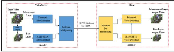
Fig. 3. Video streaming processes using SHVC
