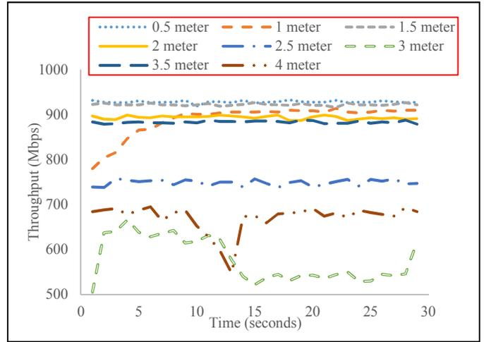
Fig. 8. The data rate of mmWave connection effected by distance
