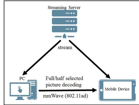
Fig. 4. The proposed system for PC offloading
